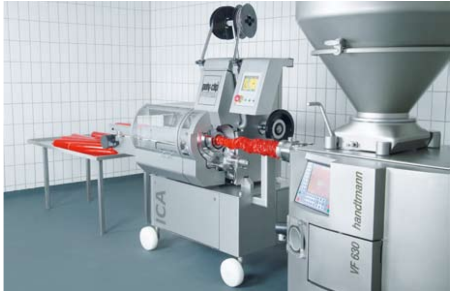
The ICA conveyor belt ensures a rapid product flow and the optional overspread guarantees perfect slack fill
