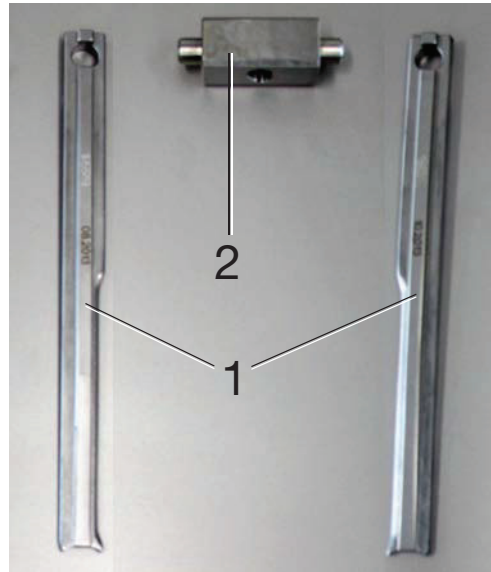
Fig. 7-10 1 Punch 2 Punch holder
