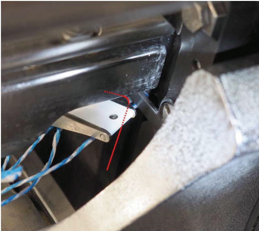
Fig. 8-5 GSA 20: Loop in correct position The red line indicates the position of the clip guide.
