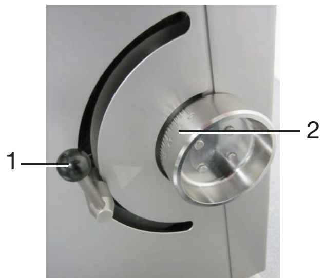
Fig. 5-20 1 Quick-locking screw 2 Separator setting scale
