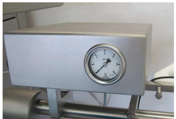
Fig. 2-2 Pneumatic casing brake control
