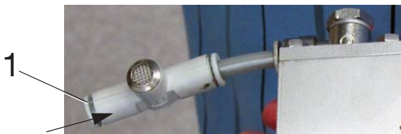
Fig. 7-32 1 Ring on the quick vent valve
