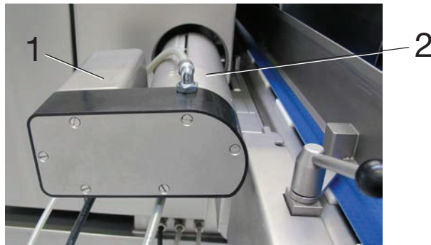
Fig. 2-5 1 Overspreading motor 2 Cylinder
